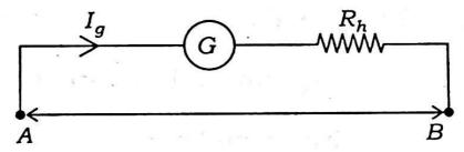
where G is the galvanometer,  $I_g$  is the current passing through the galvanometer,  $R_g$  is the galvanometer resistance,  $R_h$  is the high resistance.
