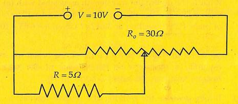
As shown in the *figure* above, a resistance of  $R = 5\Omega$  draws current from a potentiometer of total resistance  $R_o = 30\Omega$ . A voltage V = 10V is supplied to the potentiometer. What is the voltage across R when the sliding contact is in the middle of the potentiometer?
