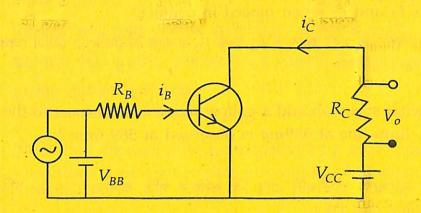
In the above circuit diagram  $V_{CC} = 8V$ ,  $V_o = 0.5V$ ,  $R_C = 800\Omega$  and  $\alpha = 0.96$ .
